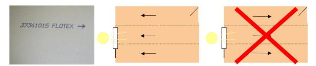
**Note:** When installing Flotex® sheet in corridors, always run arrows lengthwise. Where corridors intersect, it is recommended that a decorative border be used as a separator to avoid pattern cross match at the intersection. The arrows on the back of the sheet indicate the pile direction. Lay the sheets edge to edge, following the direction of the arrows, which should point towards the main light source, NEVER AWAY.
